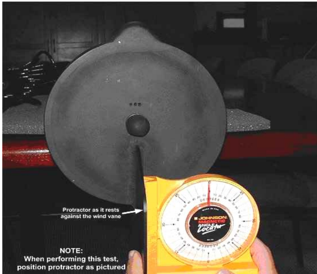
Figure 1-35 Wind Direction Test Protractor/Inclinometer/Angle Locator Position
