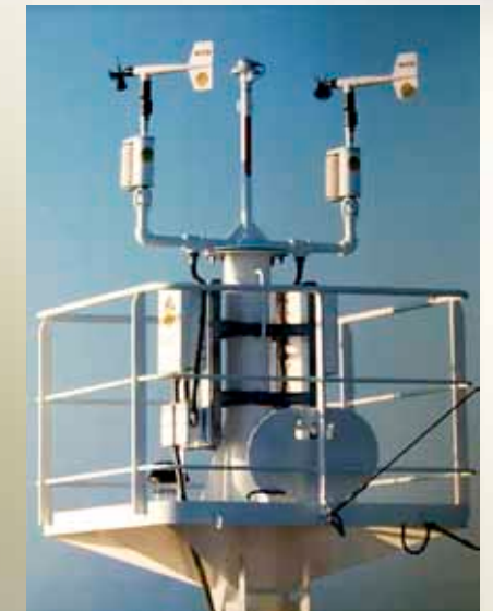
The forward sensors on the NATO "Alliance." The ship features a Coastal weather station that measures wind speed/direction/gust/sigma theta at three different points (port, starboard and aft).
